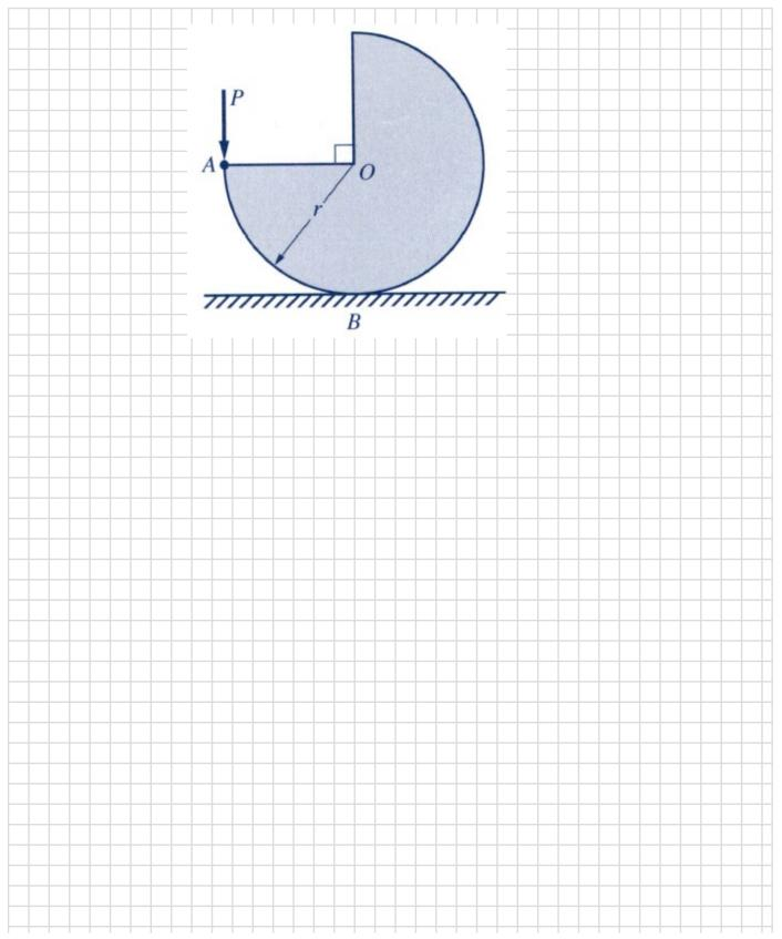
7-25 to 7-28 Refer to Figs. P7-25 to P7-28. Determine the reactions at the supports of the beams for the loading shown in each figure.
